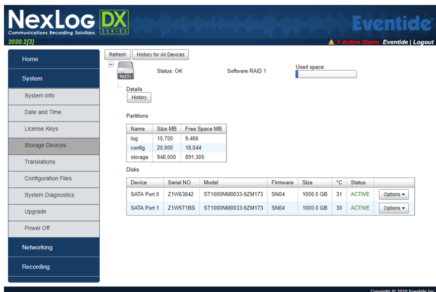
Fig. 7.5 Storage Devices: Hardware RAID-1 Example
